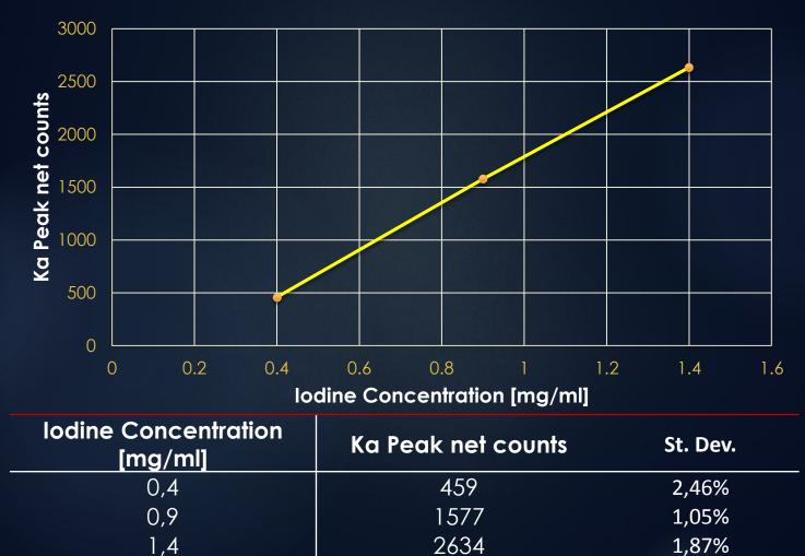
We evaluated dose on phantom in the same conditions as before, using 3 times a 0,9mg/ml iodine solution and 3 times a saline solution without iodine to fill the phantom.
