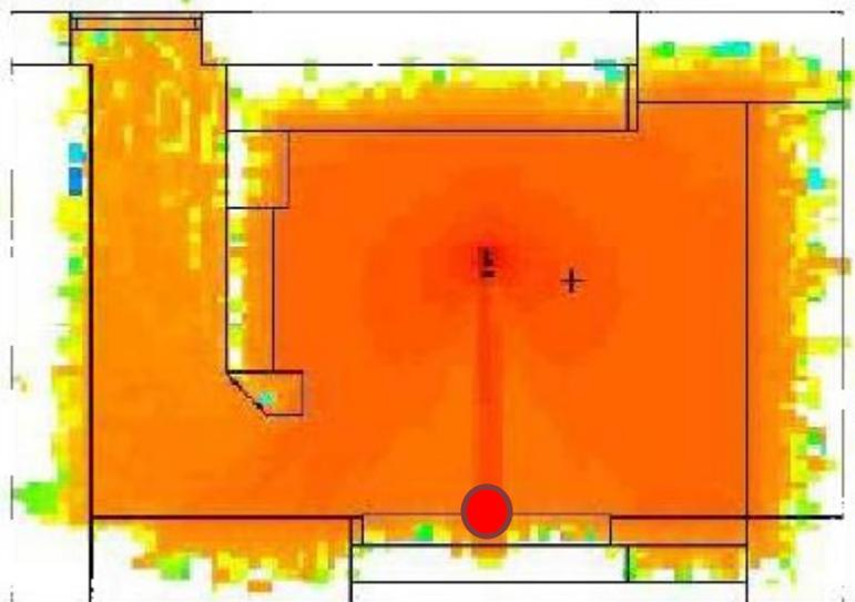
2D X-Y Visualization of the photon flux with primary beam pointed on the bunker wall
