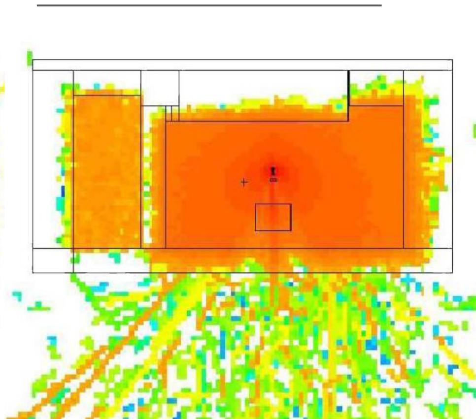
2D X-Z Visualization of the photon flux with primary beam pointed on a water phantom in the floor direction
